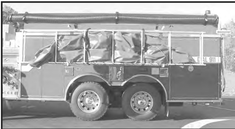
Portable tank lowered for easy removal
