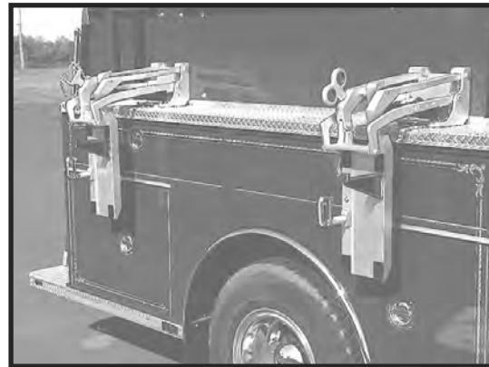
System lowered for easy ladder removal
