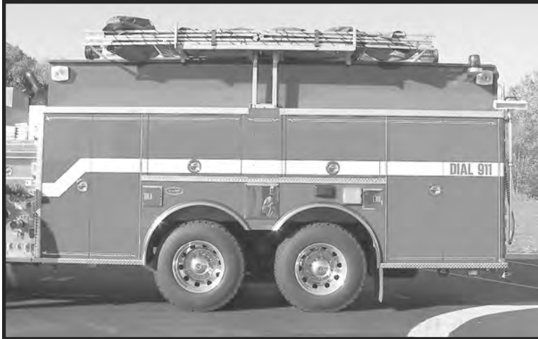
Portable tank and hard sleeve in stored position
