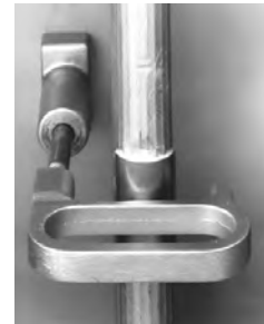
Rung protector installed showing proper placement.
