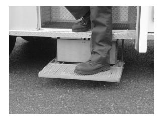
Powered by a single 12-volt electric actuator. Includes a patent pending in-line locking mechanism to hold the extended step rigidly in place.
