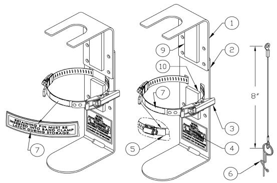
12 1/4" x 3" x 4 1/8" 13 3/4" x 3" x 4 1/8" Dimensions do not include overall dimensions of the fire extinguisher.
