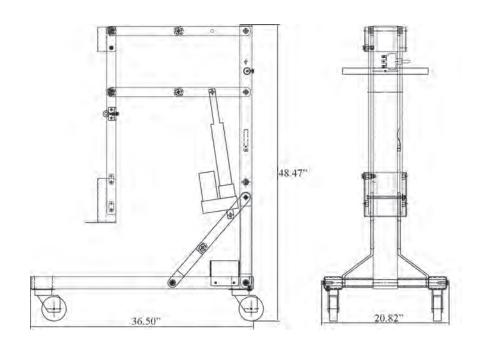
The Zico Cylinder Lift raises and lowers "M" through "J" cylinders. Unit has a maximum lifting capacity of 200 lbs.
