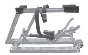
2. Assemble the horizontal legs by raising the right hand and left hand legs separately. Attaching them to the forward brace, using (1) 3/8-16" x 4" hex head bolt, (1) 3/8-16" self locking nut, and (1) 3/8" flat washer on each side. (Note: Keep the hardware loose at this time.)
