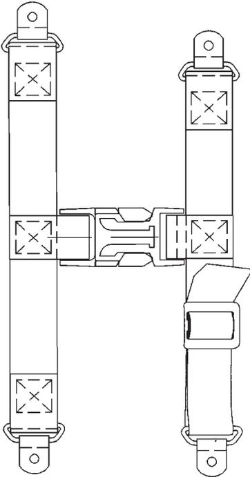
**Restraint strap prevents accidental release of SCBA air cylinder, while still providing easy access when needed.**
