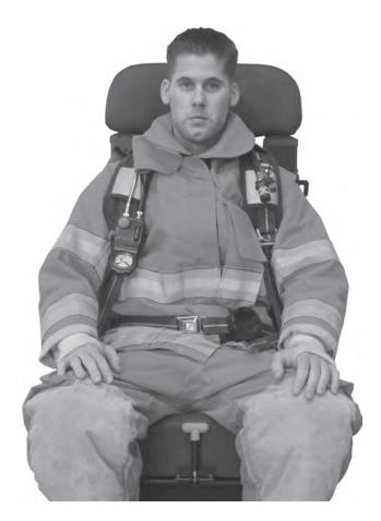
The center pull release kit allows the SCBA bracket to be released by pulling a "T" handle located on the front of the seat. The kit puts the release in an accessible location where it is not in the way of the SCBA pack straps, or the seat belt. It includes all of the parts needed to make the conversion.
