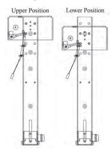
11. Insert the cable into the bottom of the "T" handle shaft. Make sure the "T" handle is in the down position then tighten the (2) 5/64" hex set screws. (There is one on the front and one on the back. The handle will need to be rotated 180° to reach the second screw.)
