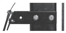
8. Take the strap clevis on the end of the cable and connect it to the Quic-Lock, in the unlocked position, as shown in the picture using (1) cotter hairpin (*Item 14*), (1) 3/16" x 1/2" Clevis Pin (*Item 16*) and (1) #10 Plain washer (*Item 15*).
