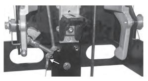
9. Feed the cable under the roller and towards the bottom of the "T" handle and pull the upper clamp on the Quic-Lock down. Secure the Quic-Lock in the locked position by pulling up on the red knob.
