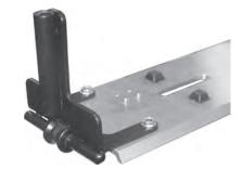
7. From the outside edge placed at the far end of the elongated slots, install the (2) 1/4-20 U nuts onto the cable plate with threads facing the channel side. (*Tapping them on lightly with a hammer makes the process easier.*)
