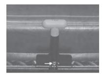
15. The center pull release should now be installed properly. Remove the shim and tighten and replace the seat cushion bolts. Make sure the Rol-Loc releases properly without the "T" handle coming out of the bracket. If it is not functioning properly, go back to step 14 and repeat.
