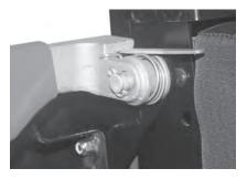
14. Feed the cable under the roller and toward the bottom of the "T" handle and insert the cable into the bottom of the "T" handle shaft. Make sure the "T" handle is in the down position, then tighten the (2) 5/64" hex set screws. (There is one in front and one on the back. The handle will need to be rotated 180° to reach the second screw.)
