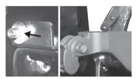
Feed the cable from the back of the Rol-Loc casting and through the cable guide as shown in the next picture. Feed the cable through the conduit until it is visible from below the release handle.
