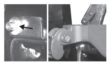
22. Feed the cable from the back of the Rol-Loc casting and through the cable guide as shown in the picture below. Feed the cable through the conduit until it is visible from below the release handle.
