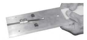
Mount the center pull release assembly (Item 1) to the channel side of the cable plate with (2) 10-32 x 3/8" screws.
