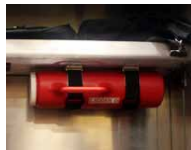
Cylinder straps on a flare container
