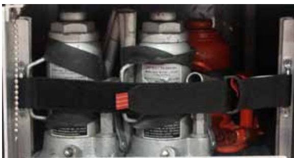
Utility straps securing jacks
