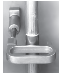
Rung protector installed showing proper placement.
