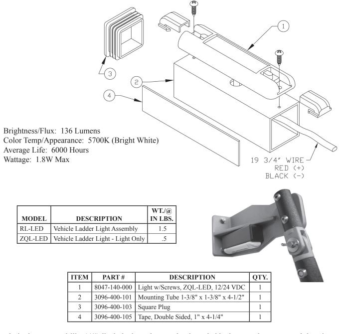
If so desired, you may drill a 1/4" dia. hole through your aluminum ladder base casting to conceal the wire. Paint the exposed edge to prevent corrosion.
