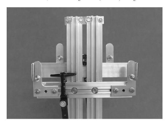
4. Adjust Rubber Strap (18) so that Strap Handle (17) grips tool handle tightly.
