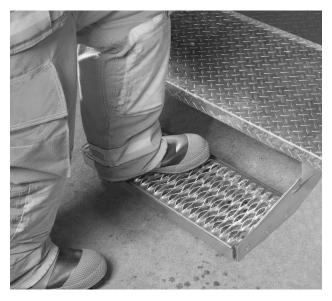
The stepping surface is 9.5" deep and is a non-skid surface to provide traction and safety. Also, it allows mud and debris to fall through rather than stay on the stepping surface.
