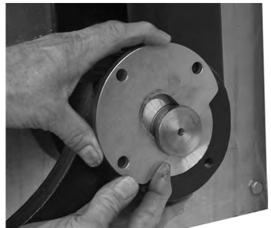
6. Slide lock plate in position and insert fasteners.
