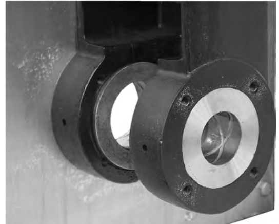
2. Base casting ears showing hole for shaft insertion.
