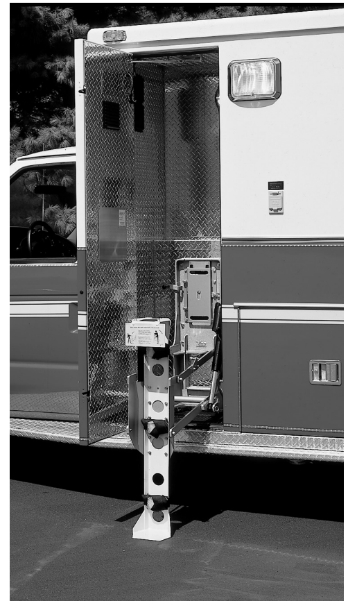
Designed specifically for "M" cylinders, this new bracket requires a mounting area 15-1/2" W x 33-1/2" H x 10-5/8" D. Minimum door opening is 12".
