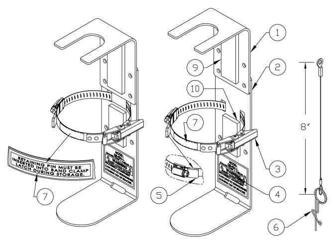
12 1/4" x 3" x 4 1/8" 13 3/4" x 3" x 4 1/8" Dimensions do not include overall dimensions of the fire extinguisher.
