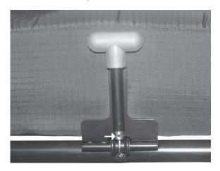
12. Loosen the 5/64" set screw in the stop barrel and pull the "T" handle until the Quic-Lock unlocks. Stop pulling the "T" handle after it unlocks and hold it in that position. Make sure that the barrel is as low as it can go, then tighten the set screw.
