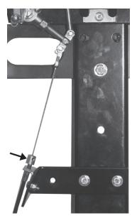
13. The center pull release should now be installed properly. Check to make sure that it releases the Quic-Lock properly with the "T" handle coming out of the bracket. If this is an issue, begin with step 11 again and follow to the end.
