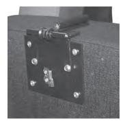
4. Attach the conduit assembly 47" (3) to the mounting bracket using a 6mm push nut (an extra push nut, Item 5, is provided in the event the first is damaged during installation).
