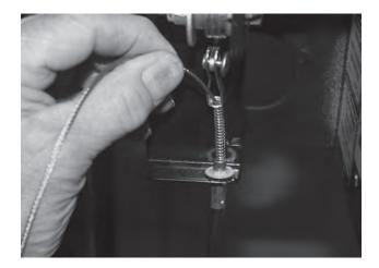
8. Feed the cable under the roller and toward the bottom of the "T" handle and insert the cable into the bottom of the "T" handle shaft. Make sure the "T" handle is in the down position, then tighten the two 5/64" hex set screws (there is one front and one back; the handle will need to be rotated 180 degrees to reach the second screw).
