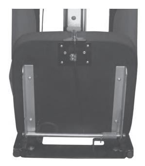
The center pull release kit allows the SCBA bracket to be released by pulling a "T" handle located on the front of the seat. The kit puts the release in an accessible location where it is not in the way of the SCBA pack straps or the seat belt. It includes all of the parts needed for setup.
