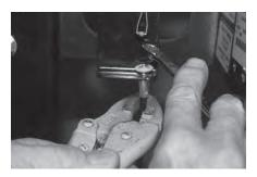
5. The end of the conduit (3) with the crimped fitting can now be routed between the seat and the hinge rod and up to and through the access hole to engage the pull release bracket attached to the top strap.
