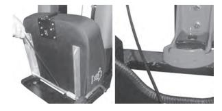
6. Feed the non-crimped end of the conduit through the clamps, push it even with the end of the plate, and tighten the clamps.
