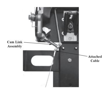
6. Confirm that the release is functioning properly to finalize install.
