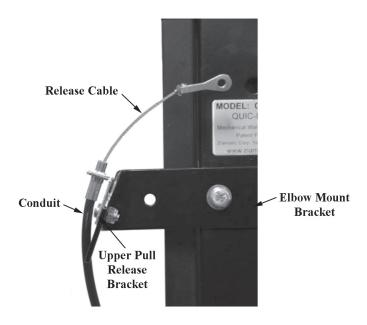
4. Attach the Pull Release Bracket (4), with Yellow Tubing (2) and Release Cable (1) to desired position on the seat frame. Drill two holes with a #19 drill (.166). Use two 10-32 x 3/8" threaded forming screws to attach the bracket to the seat frame. Note: A thicker seat frame may require a #18 drill bit (.169). Carefully run the cable and conduit around the seat and bracket without causing kinks in the cable or interference with the bracket's function.
