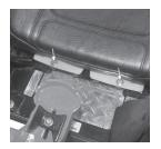
2. Lay out and drill (2) 25/64" holes on the center of the brace spaced 2-1/4" apart.
