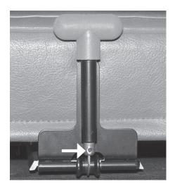
17. Loosen the 5/64" set screw in the stop barrel and pull the "T" handle until the Quic-Lock unlocks. Stop pulling the "T" handle after it unlocks and hold it in that position. Make sure that the barrel is as low as it can go, then tighten the set screw.
