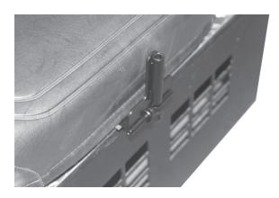
11. Mount the release bracket (Item 12) to the Quic-Lock using (2) 1/4-20 x 3/4" screws (Item 18) and (2) 1/4" plain washer (Item 19).
