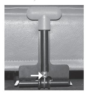
16. Loosen the 5/64" set screw in the stop barrel and pull the "T" handle until the Quic-Lock unlocks. Stop pulling the "T" handle after it unlocks and hold it in that position. Make sure that the barrel is as low as it can go, then tighten the set screw.
