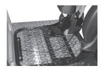
7. From the channel side of the cable plate, feed the conduit and cable through the center slot and under the clamps. Push the conduit even with the end of the cable plate and tighten the clamps.
