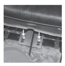
10. Let the seat cushion go all the way down and push the release assembly into the chosen location.
