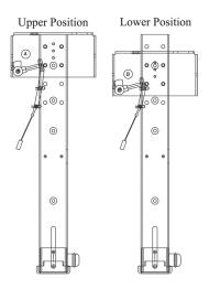
16. Insert the cable into the bottom of the "T" handle shaft. Make sure the "T" handle is in the down position then tighten the (2) 5/64" hex set screws. (There is one on the front and one on the back.) The handle will need to be rotated 180° to reach the second screw.
