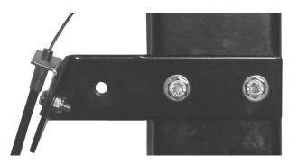
12. Take the strap clevis on the end of the cable and connect it to the Quic-Lock, in the unlocked position, as shown in the picture using (1) cotter hairpin (Item 20), (1) 3/16" x 1/2" clevis pin (Item 22) and (1) #10 plain washer (Item 21).
