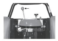
15. If the upper bracket of the Quic-Lock is in the top position, the cable is the proper length. If the Quic-Lock upper bracket is in the lower position, then 2 inches must be trimmed off the cable before attaching it to the "T" handle.
