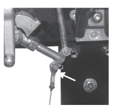
13. Feed the cable under the roller and towards the bottom of the "T" handle and pull the upper clamp on the Quic-Lock down. Secure the Quic-Lock in the locked position by pulling up on the red knob.
