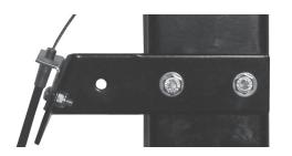
13. Take the strap clevis on the end of the cable and connect it to the Quic-Lock, in the unlocked position, as shown in the picture using (1) cotter hairpin (Item 20), (1) 3/16" x 1/2" clevis pin (Item 22) and (1) #10 plain washer (Item 21).
