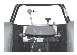
14. If the upper bracket of the Quic-Lock is in the top position, the cable is the proper length. If the Quic-Lock upper bracket is in the lower position, then 2 inches must be trimmed off the cable before attaching it to the "T" handle.
