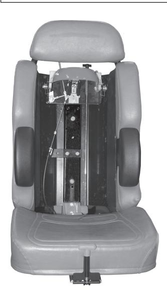
The center pull release kit allows the SCBA bracket to be released by pulling a "T" handle located on the front of the seat. The kit puts the release in an accessible location where it is not in the way of the SCBA pack straps, or the seat belt. It includes all of the parts needed to make the conversion.
