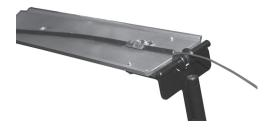
8. Install the conduit and cable plate under the front of the seat frame and springs keeping it above the mounting frame and the cross brace.
