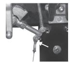
14. Feed the cable under the roller and towards the bottom of the "T" handle and pull the upper clamp on the Quic-Lock down. Secure the Quic-Lock in the locked position by pulling up on the red knob.
