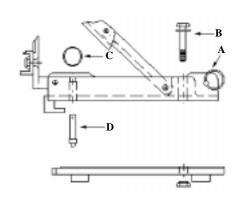
(C). 4. Push out lock pin (D). Now reverse steps 4 to 1 for right side assembly.
