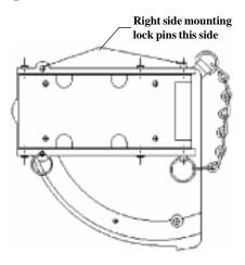
Assembly shown for left side of vehicle mounting. For right side mounting, move lock pins to opposite side. See lock pin removal.
