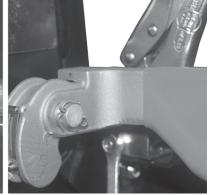
22. Feed the cable from the back of the Rol-Loc casting and through the cable guide as shown in the picture below. Feed the cable through the conduit until it is visible from below the release handle
