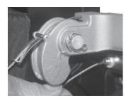
14. Insert an approximate 1/16" shim under the top clamp to alleviate tension on the cable.
