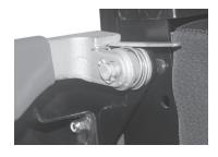
15. Feed the cable under the roller and toward the bottom of the "T" handle and insert the cable into the bottom of the "T" handle shaft. Make sure the "T" handle is in the down position, then tighten the (2) 5/64" hex set screws. (There is one in front and one on the back. The handle will need to be rotated 180° to reach the second screw.)
