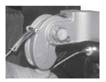
13. Insert an approximate 1/16" shim under the top clamp to alleviate tension on the cable.
