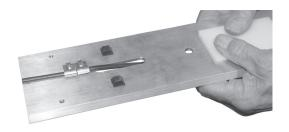
6. Mount the center pull release assembly (Item 1) to the channel side of the cable plate with (2) 10-32 x 3/8" screws.
