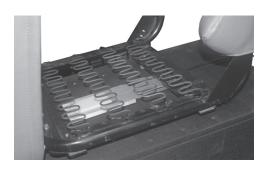
9. Allow the seat cushion to rest back down far enough to start 1/4" x 3/4" hex screws with flat washers through the (2) 9/32" holes in the rear seat mount into the U nuts. **Do not tighten.**
