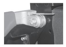
14. Feed the cable under the roller and toward the bottom of the "T" handle and insert the cable into the bottom of the "T" handle shaft. Make sure the "T" handle is in the down position, then tighten the (2) 5/64" hex set screws. (There is one in front and one on the back. The handle will need to be rotated 180° to reach the second screw.)
