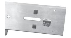
5. From the channel side of the cable plate, pass the non-crimped end of the conduit through the center slot and under the clamps. Push the conduit even with the end of the cable plate and tighten the clamps.
