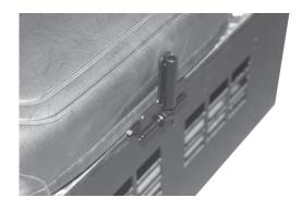
10. Route the conduit up to and through the access hole on the Rol-Loc's upper bracket to engage the pull release bracket attached to the top strap.
