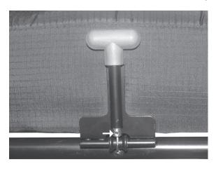
12. The center pull release should now be installed properly. Remove the shim and check to make sure that it releases the Rol-Loc properly without the "T" handle coming out of the bracket. If this is an issue, begin with step 11 again and follow to the end.
