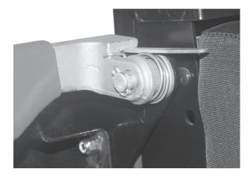
11. Feed the cable under the roller and toward the bottom of the "T" handle and insert the cable into the bottom of the "T" handle shaft. Make sure the "T" handle is in the down position, then tighten the (2) 5/64" hex set screws. (There is one on the front and one on the back. The handle will need to be rotated 180° to reach the second screw.)
