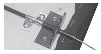
7. Hold the "T" handle and mounting bracket (*Item 1*) to the front of the seat so that it is flush on the front of the seat. Once in the proper position, secure it using (2) #10 wood screws that are included in the bag with Item 1.
