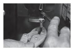
5. The end of the conduit (3) with the crimped fitting can now be routed between the seat and the hinge rod and up to and through the access hole to engage the pull release bracket attached to the top strap.
