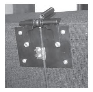
7. Attach your new cable (2) through the strap fork. Slide your new spring (7) onto the cable.
