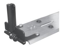
10. Install the (2) 1/4-20 U nuts onto the Cable Plate with threads facing the channel side, placed at the far end of the elongated slots. (*Tapping them on lightly with a hammer makes the process easier.*)
