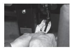
4. Remove the conduit assembly and slide the cable assembly out through the top of the strap fork. The spring should now be loose.
