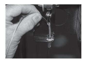
17. Slide the Cable Assembly (*Item 3*) through the Conduit (*Item 4*). It will extend out under the roller on the Center Pull Release.
