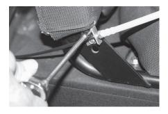
3. Using vise grips and a pry tool, carefully remove the push nut from the black mounting bracket that secures the black conduit assembly on your EZ-LOC bracket.
