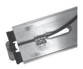
12. With the channel down, pass the Cable Plate (*Item 2*) with attached conduit under the front of the seat cushion, the springs, and the rear seat mount. Direct the crimped end of the conduit into the vicinity of the mounting bracket.
