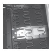
14. Let the seat cushion go all the way down and push the Cable Release Assembly (*Item 1*) against the cushion, allowing room for proper operation. Once in place, lift the cushion just enough to tighten the (2) screws holding the Cable Plate (*Item 2*) in place.
