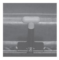
20. The Center Pull Release should now be installed properly. Check to make sure that it releases the EZ-LOC properly and returns to the locked, fully-engaged position smoothly.
