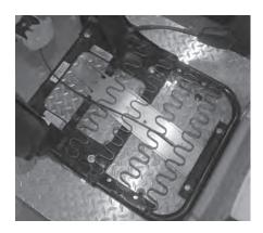
12. Allow the seat cushion to rest back down far enough to start  $1/4-20 \ge 3/4$ " hex screws with 1/4-20 flat washers through the slots in the Cable Plate and into the U nuts. (Hand tighten two turns.)
