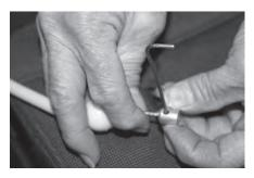
2. Remove the bracket holding the yellow pull release stalk (10" yellow tube) from your seat.
