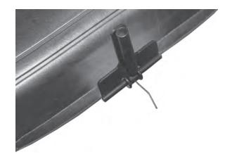
17. Feed the cable under the roller and toward the bottom of the "T" handle and pull the Top Clamp on the EZ-LOC down. Check that the Serrated Latch Assembly is fully engaged.
