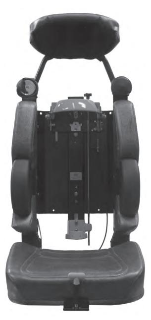
Model QM-EZL-CPR-TS is made for the EZ-LOC SCBA bracket mounted in a Bostrom Tanker Series seat. For additional models and other bracket/seat combinations please contact us at 1-800-711-FIRE. The center pull release kit allows the SCBA bracket to be released by pulling a "T" handle located on the front of the seat. The kit puts the release in an accessible location where it is not in the way of the SCBA pack straps or the seat belt. It includes all of the parts needed for setup.
