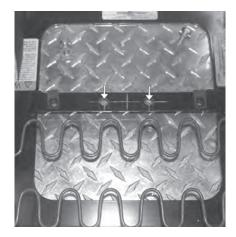
7. Insert the (2) U nuts (*Item 11*) into the holes, threads down.
