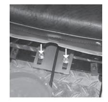
13. Let the seat cushion go all the way down and push the release assembly into the chosen location. Once in place, raise the cushion post enough to tighten the (2) screws holding the cable plate in place.
