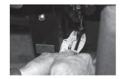
4. Remove the conduit assembly and slide the cable assembly out through the top of the strap fork. The spring should now be loose.
