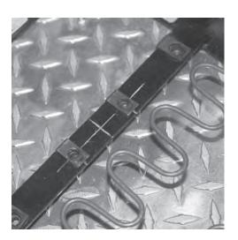
8. Mount the conduit clamps (*Item 5*) to the flat side of the cable plate (*Item 2*) with the 8-32 x 3/8" screws (*Item 7*). At this time, only hand tighten two full turns.
