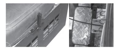
14. Attach your new conduit assembly 47" (*Item 4*) to the mounting bracket using a 6mm push nut (an extra push nut, *Item 12*, is provided in the event the first is damaged during installation).
