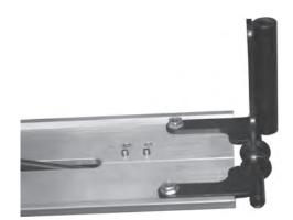
11. Install the conduit and Cable Plate under the front of the seat frame and springs, keeping it above the mounting frame and cross brace.
