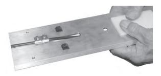
10. Mount the center pull release assembly (*Item 1*) to the channel side of the cable plate with (2) 10-32 x 3/8" screws.
