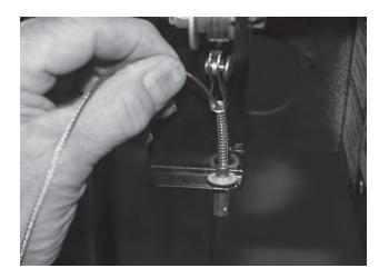
16. Slide the cable assembly (*Item 3*) through the conduit (*Item 4*). Look for it to extend out from under the roller on the Pull Release Assembly.
