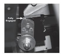
15. Insert the cable into the bottom of the "T" handle shaft. Make sure the "T" handle is in the down position then tighten the (2) 5/64" hex set screws. (There is one on the front and one on the back. The handle will need to be rotated 180° to reach the second screw.)
