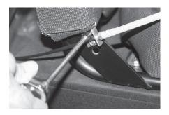
3. Using vise grips and a pry tool, carefully remove the push nut from the black mounting bracket that secures the black conduit assembly.
