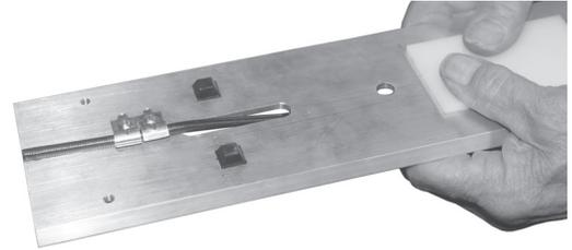
6. Mount the center pull release assembly (Item 1) to the channel side of the cable plate with (2) 10-32 x 3/8" screws.
