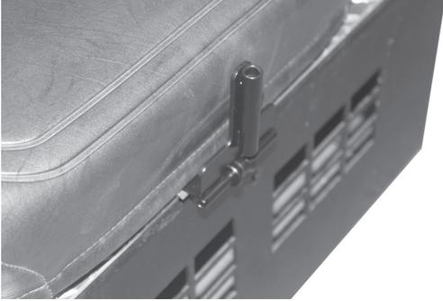
10. Route the conduit up to and through the access hole on the Rol-Loc's upper bracket to engage the pull release bracket attached to the top strap.
