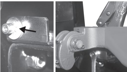
13. Feed the cable from the back of the Rol-Loc casting and through the cable guide as shown in the next picture. Feed the cable through the
