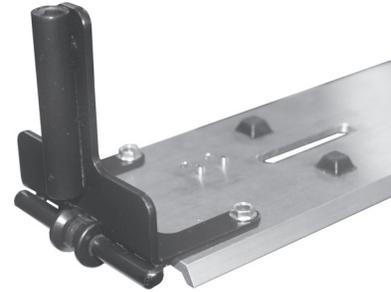
7. From the outside edge placed at the far end of the elongated slots, install the (2) 1/4-20 U nuts onto the cable plate with threads facing the channel side. (Tapping them on lightly with a hammer makes the process easier.)
