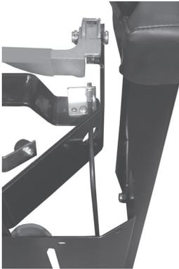
11. Hold crimped conduit end into the bracket from behind and push spring retaining nut onto the conduit end. A set of vise grips and a box wrench are suggested.
