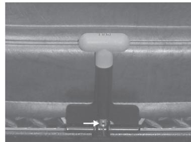
15. The center pull release should now be installed properly. Remove the shim and tighten and replace the seat cushion bolts. Make sure the Rol-Loc releases properly without the "T" handle coming out of the bracket. If it is not functioning properly, go back to step 14 and repeat.
