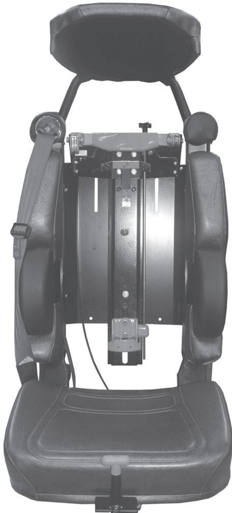
The center pull release kit allows the SCBA bracket to be released by pulling a "T" handle located on the front of the seat. The kit puts the release in an accessible location where it is not in the way of the SCBA pack straps or the seat belt. It includes all of the parts needed to make the conversion.
