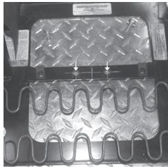
3. Insert the (2) U nuts (Item 10) into the holes, threads down.
