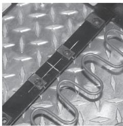
4. Mount the conduit clamps (Item 5) to the flat side of the cable plate (Item 2) with the 8-32 x 3/8" screws (Item 7). **Do not tighten.**
