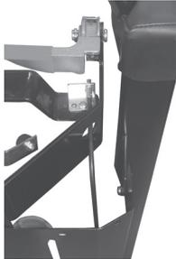
12. Hold crimped conduit end into the bracket from behind and push spring retaining nut onto the conduit end. A set of vise grips and a box wrench are suggested.
