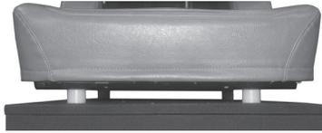
2. Remove the (2) bolts holding the rear of the seat cushion down to the cross brace, then flip the cushion up.
