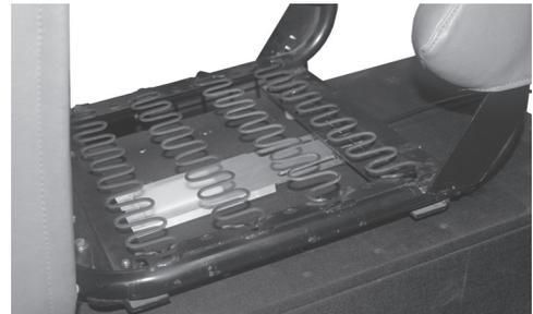
9. Allow the seat cushion to rest back down far enough to start 1/4" x 3/4" hex screws with flat washers through the (2) 9/32" holes in the rear seat mount into the U nuts. **Do not tighten.**
