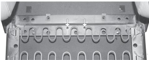
4. Mount the conduit clamps (Item 5) to the channel side of the cable plate (Item 2) with the 8-32 x 3/8" screws (Item 7). At this time, only hand tighten two full turns.
