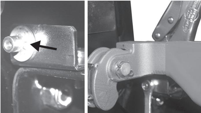
22. Feed the cable from the back of the Rol-Loc casting and through the cable guide as shown in the picture below. Feed the cable through the conduit until it is visible from below the release handle.
