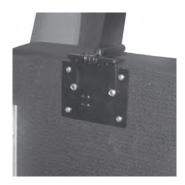
3. Mount the conduit clamps (Item 5) to the plate with the 8-32 x 3/8" screws (Item 7). Do not tighten.
