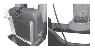
5. Hold crimped conduit end into the bracket from behind and push spring retaining nut onto the conduit end. A set of vise grips and a box wrench are suggested.
