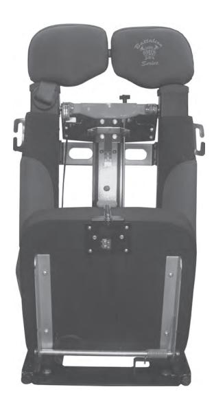
The center pull release kit allows the SCBA bracket to be released by pulling a "T" handle located on the front of the seat. The kit puts the release in an accessible location where it is not in the way of the SCBA pack straps, or the seat belt. It includes all of the parts needed to make the conversion.
