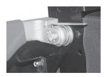
9. Feed the cable under the roller and toward the bottom of the "T" handle and insert the cable into the bottom of the "T" handle shaft. Make sure the "T" handle is in the down position, then tighten the (2) 5/64" hex set screws. (There is one front and one on the back. The handle will need to be rotated 180° to reach the second screw.)
