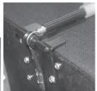
10. Secure the conduit (Item 4) with the cable tie (Item 9) off to the side, so that it will not interfere with the SCBA when being stored or removed.
