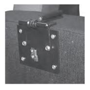
4. The end of the conduit (Item 4) with the crimped fitting can now be routed between the seat and the hinge rod and up to and through the access hole to engage the pull release bracket attached to the top strap.
