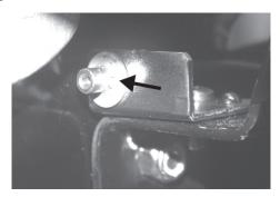
3. Feed the cable housing from the rear hole into the cable housing bracket. Use a push nut (*Item 5*) to attach it to the bracket. A pair of vice grips and a 5/16" box wrench is suggested for this process.
