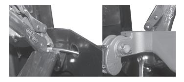
4. Feed the cable from the back of the Rol-Loc casting and feed it through the cable guide as shown in the picture below. Feed the cable through until it is visible from the end of the conduit.
