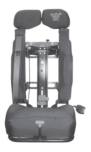
The center pull release kit allows the SCBA bracket to be released by pulling a "T" handle located on the front of the seat. The kit puts the release in an accessible location where it is not in the way of the SCBA pack straps, or the seat belt. It includes all of the parts needed to make the conversion.
