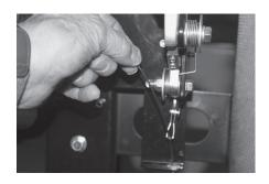
5. Now that all of the Universal Pull Release components are removed, begin your Center Pull Release installation by attaching your new conduit assembly 47" (*Item 3*) to the mounting bracket using a 6mm push nut (an extra push nut, *Item 5*, is provided in the event the first is damaged during installation).
