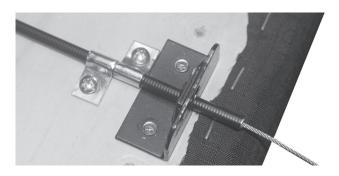
11. Hold the "T" handle and mounting bracket (*Item 1*) to the front of the seat so that it is flush on the front of the seat. Once in the proper position secure it using (2) #10 wood screws that are included in the bag with Item 1.
