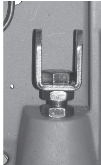
FIGURE 1 ACTUATOR YOKE ADJUSTMENT (See Section VI. C. 1.)
