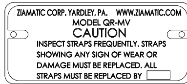
3030-135-140 Model/Caution Tag with replacement date in the bottom right corner.
