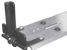
6. From the outside edge placed at the far end of the elongated slots, install the (2) 1/4-20 extruded U nuts onto the cable plate with threads facing the channel side. (Tapping on them lightly with a hammer makes the process easier.)
