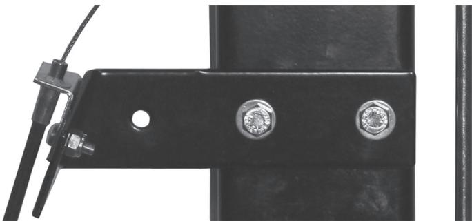
12. Take the strap clevis on the end of the cable and connect it to the Quic-Lock, in the unlocked position, as shown in the picture using (1) cotter hairpin (Item 20), (1) 3/16" x 1/2" clevis pin (Item 22) and (1) #10 plain washer (Item 21).
