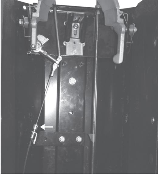
18. The center pull release should now be installed properly. Check to make sure that it releases the Quic-Lock properly without the "T" handle coming out of the bracket. If this is an issue, begin with step 11 again and follow to the end.
