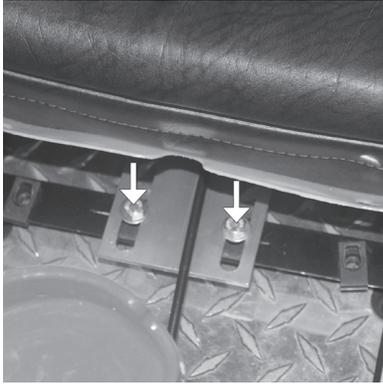
10. Let the seat cushion go all the way down and push the release assembly into the chosen location. Once in place, tighten the (2) screws holding the cable plate in place.
