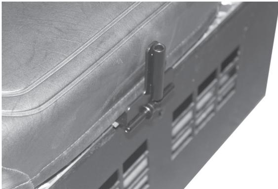
11. Mount the release bracket (Item 12) to the Quic-Lock using (2) 1/4-20 x 3/4" screws (Item 18) and (2) 1/4" plain washer (Item 19).
