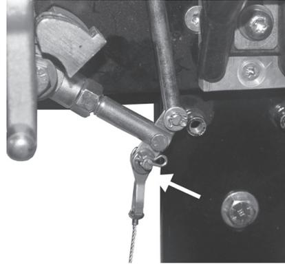
13. Feed the cable under the roller and towards the bottom of the "T" handle and pull the upper clamp on the Quic-Lock down. Secure the Quic-Lock in the locked position by pulling up on the red knob.
