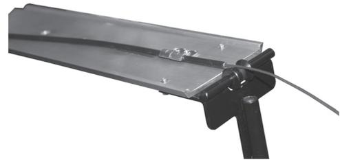
8. Install the conduit and cable plate under the front of the seat frame and springs keeping it above the mounting frame and the cross brace.
