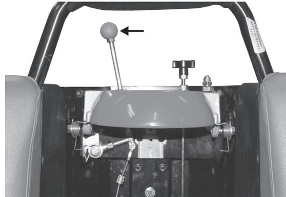
14. If the upper bracket of the Quic-Lock is in the top position, the cable is the proper length. If the Quic-Lock upper bracket is in the lower position, then 2 inches must be trimmed off the cable before attaching it to the "T" handle.
