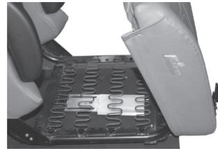
10. Allow the seat cushion to rest back down far enough to start 1/4" x 3/4" hex screws with flat washers through the (2) 9/32" holes in the rear seat mount into the U nuts. (Do not tighten.)
