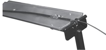
9. Lift the cushion and feed the cable plate, channel down, with the attached conduit and cable under the front seat mount, springs and the rear seat mount.
