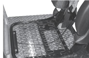
7. From the channel side of the cable plate, feed the conduit and cable through the center slot and under the clamps. Push the conduit even with the end of the cable plate and tighten the clamps.
