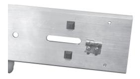
9. From the channel side of the Cable Plate, pass the non-crimped end of the conduit through the center slot and under the clamps. Push the conduit even with the end of the Cable Plate and tighten the clamps.
