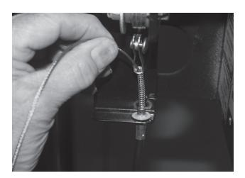
16. Slide the cable assembly (*Item 3*) through the conduit (*Item 4*). Look for it to extend out from under the roller on the Pull Release Assembly.
