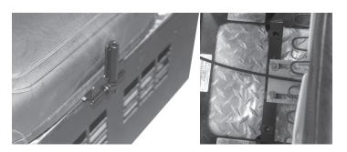
14. Attach your new conduit assembly 47" (*Item 4*) to the mounting bracket using a 6mm push nut (an extra push nut, *Item 12*, is provided in the event the first is damaged during installation).
