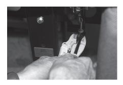
4. Remove the conduit assembly and slide the cable assembly out through the top of the strap fork. The spring should now be loose.
