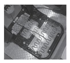
12. Allow the seat cushion to rest back down far enough to start 1/4-20 x 3/4" hex screws with 1/4-20 flat washers through the slots in the Cable Plate and into the U nuts. (Hand tighten two turns.)
